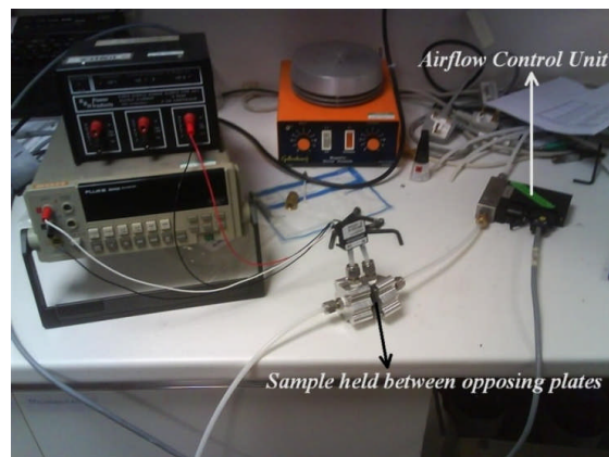
Figure 2.19 – Mass flow meter setup for porosity estimation
