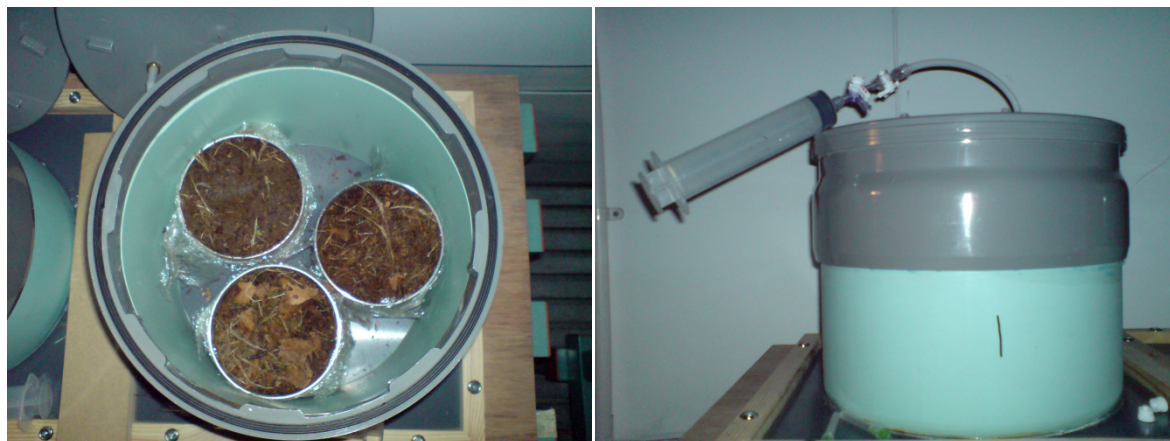
Figure 2.3: Closed-chamber set-up for the measurement of net CH 4 fluxes.
