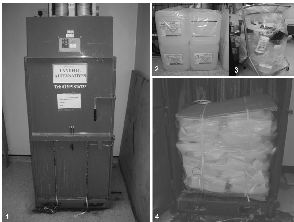
Figure 13. The baling process during the disposal of cardboard and plastic acid containers.
