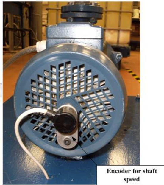
Figure 4-19 Position of encoder for shaft speed
