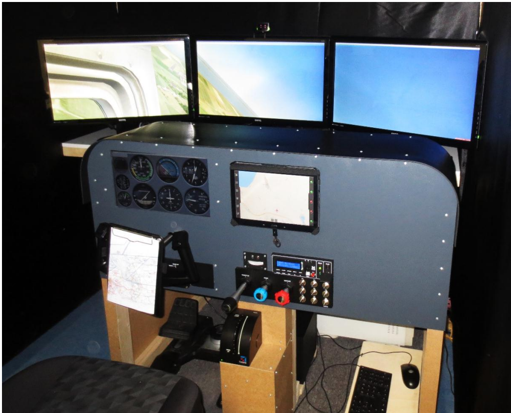
Figure 5-6. Mock-up of the flight simulator, replicating a Cessna 172S.
