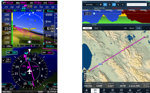
Figure 2.2.: Electronic flight instrumentation with navigational information. PFD (left) with synthetic vision and a HSI on the bottom (Garmin G3X). Ipad with map (right) and vertical situation display (ForeFlight). Source: [57; 61].
