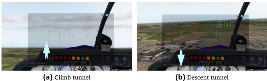
Figure 3.8.: Flight Tunnel display format prototype. Early implementation in Laminar Research 'X-plane 9.70' for demonstration. [139]
