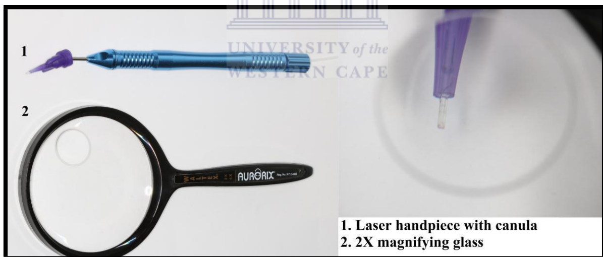
Figure 5: Correctly cleaved fiber assessed under 2X magnification.
