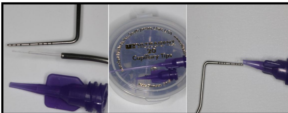
Figure 8: Illustration of how canula was calibrated for the laser fiber
