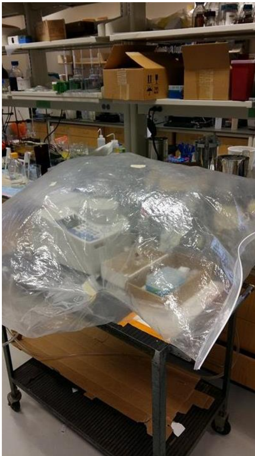
Figure 15: The apparatus used to exclude atmospheric oxygen to monitor the of the rates of reaction of the tocopheryl quinones with NAC by UV/Vis spectroscopy. The UV/Vis spectrophotometer is inside the bag with the necessary reagents for the reaction and the bag was filled with N 2 gas.
