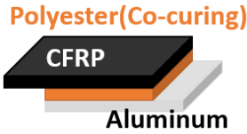
Figure 35. Schematic diagram of the CFRP-aluminum single-lap co-cured joints.
