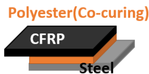
Figure 33. Schematic diagram of the CFRP-steel single-lap co-cured joints.
