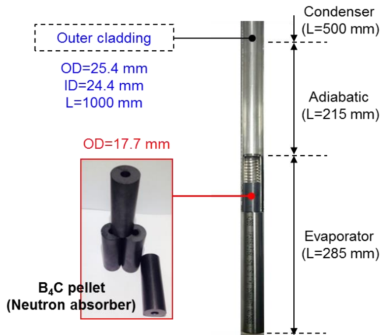
Fig 2-3. Composition and dimensions of the test section
