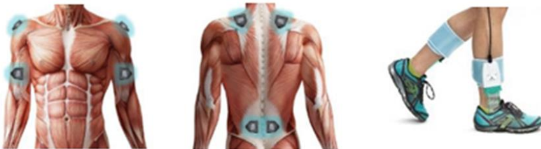
Figure 13. The placements of EMG and insole sensors
