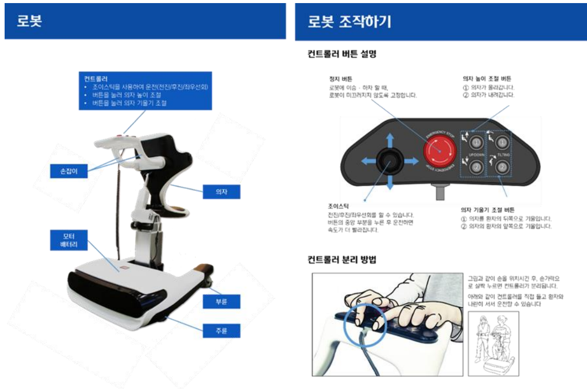
Figure 11. Illustration of CarryBot in the user manual included description of each components, controller button, and operation methods.
