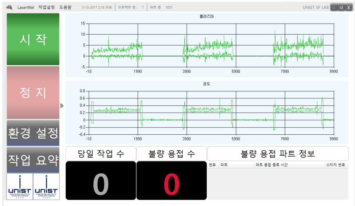
Figure 5-8 Another version of developed monitoring software for production environment
