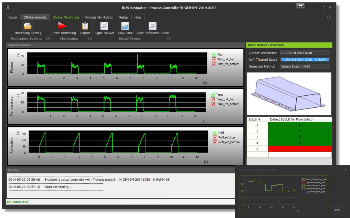
Figure 5-5 A main panel of the developed monitoring software
