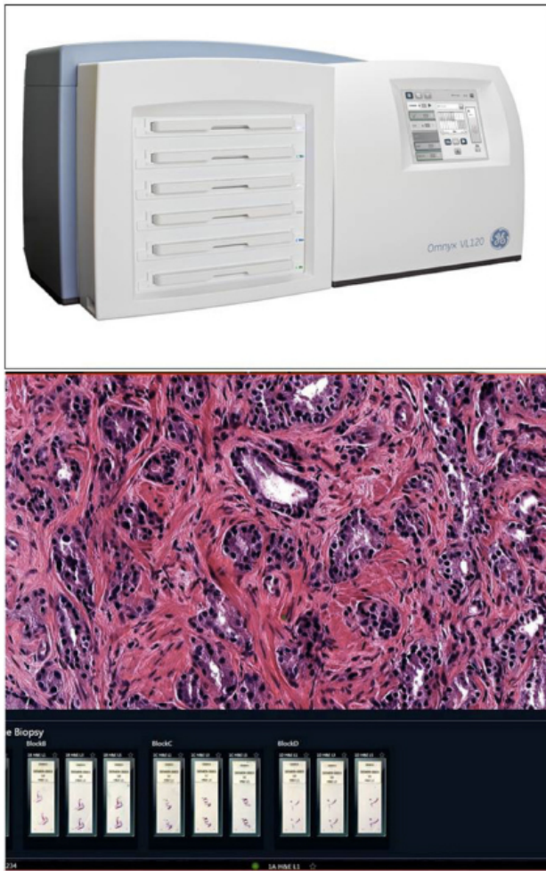
Figure 11. Left: Example of a whole slide imaging scanner (top) and PACS from the same manufacturer (Omnyx®, bottom). Virtual slide composed of multiple image acquisitions from a physical glass slide. Right: List of currently available commercial whole slide scanners. Modified from Farahani et al (170), reprinted under a creative commons license.
