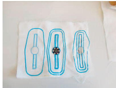
Fig.1 Examples of a 3D printed electronic circuits
