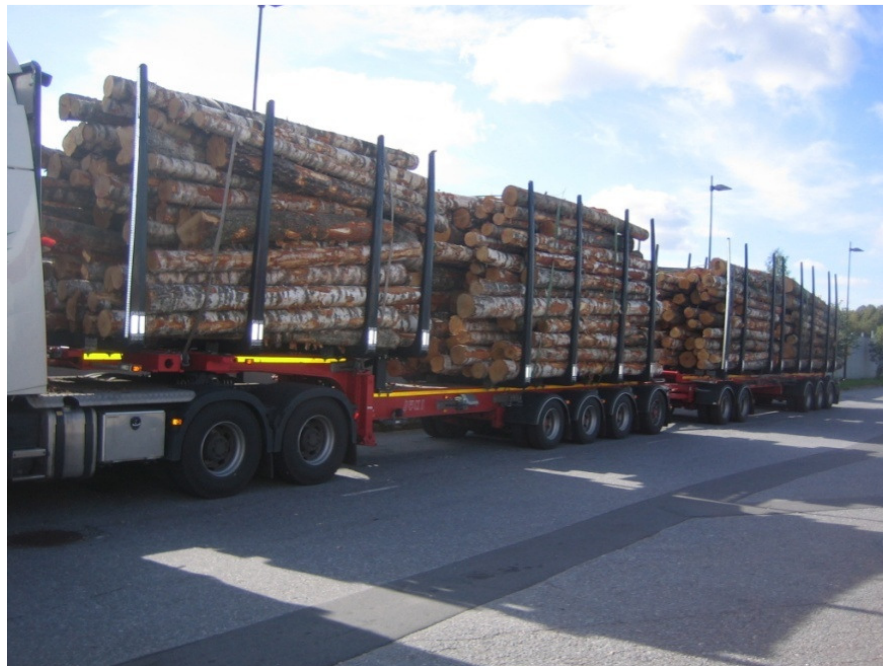
Figure 2. Maximum payload in 90 t vehicle combination (photo: T. Palander)
