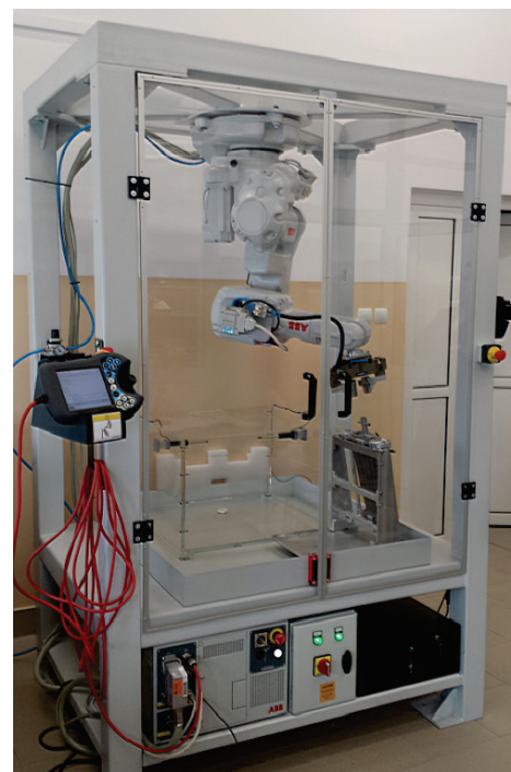
Figure 10 Robotic vane thickness measurement stand
