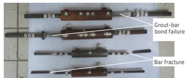
Figure 5. Two observed failure modes
