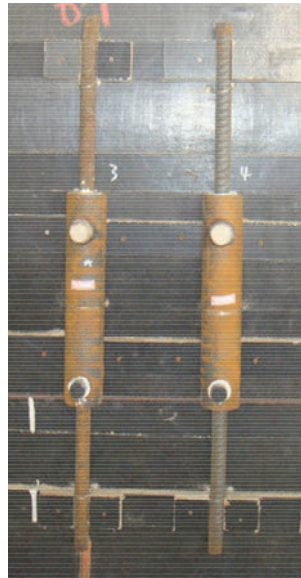
Figure 3. Grouted splice specimens
