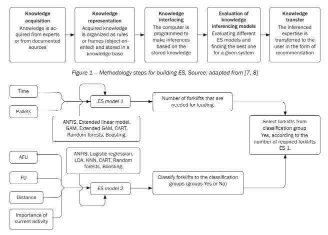
Figure 2 – Building structure of ESs
