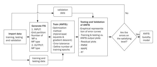
Figure 3 – Methodology steps for building the ANFIS model
