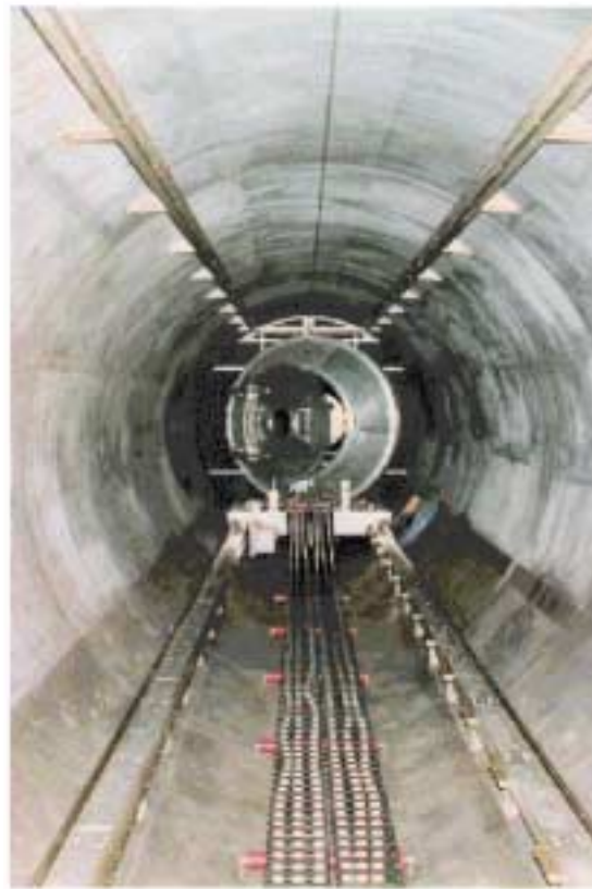
Figure 83: View of D22 multidetector in 20m long vacuum chamber.
