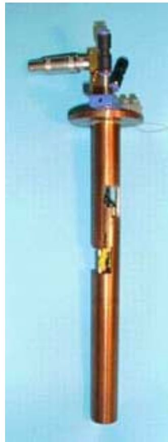
Figure 18: Peltier cooled NMR probe.
