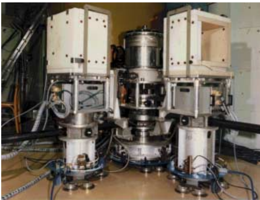
Figure 79: View of D4B neutron diffractometer, showing sample vacuum chamber and the two multidetector housings.
