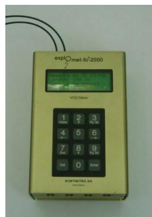
Figure 2. Electronic timer "Explomet-Fo-2000"
