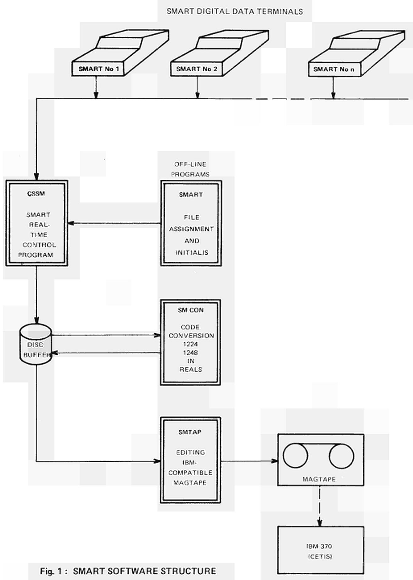
Fig. 1 : SMART SOFTWARE STRUCTURE
