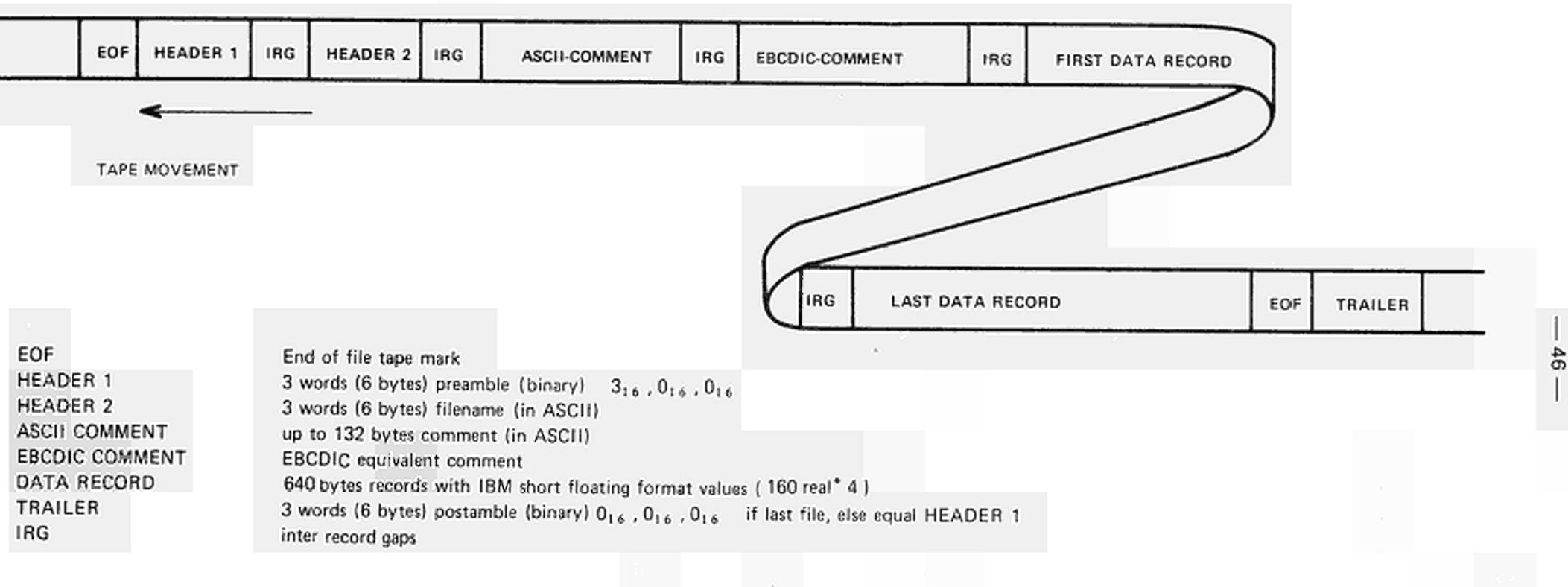
Fig. 8 : SPC - 16 – IBM COMPATIBLE TAPE FORMAT (9 track tape record)
