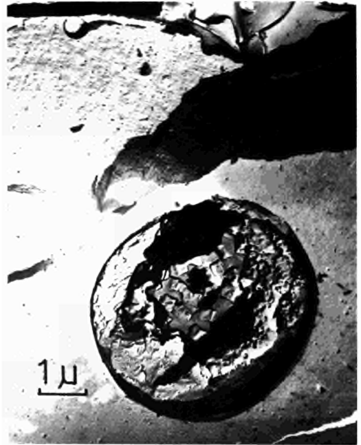
Fig. 6 : Pore containing solid fission products
