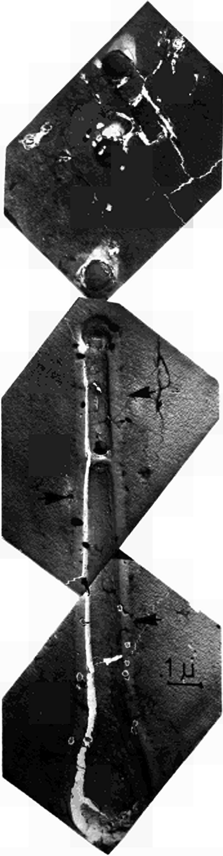
Fig. 9 : Scission of a pipe-shaped pore under surface tension forces. The etching reveals the presence of contaminants on its surface (arrows)
