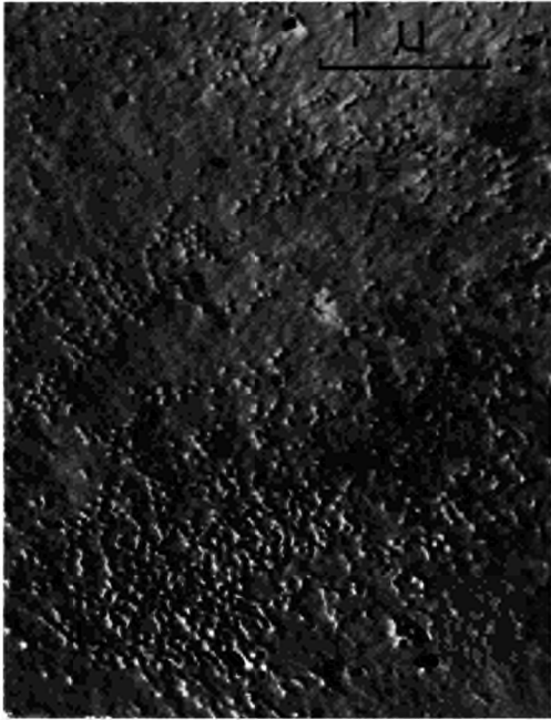
Fig. 5 : Small precipitates revealed by slight CV etching. Their contrast is here reversed, compared with that of the bubbles
