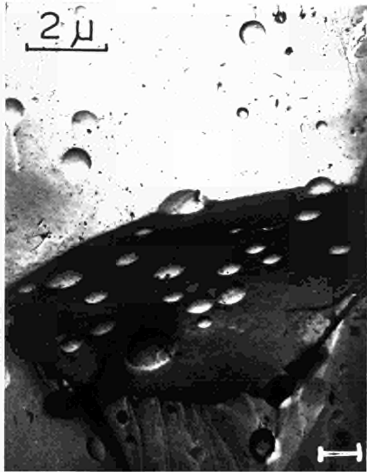
Fig. 13 : Intergranular porosity observed in a fracture surface
