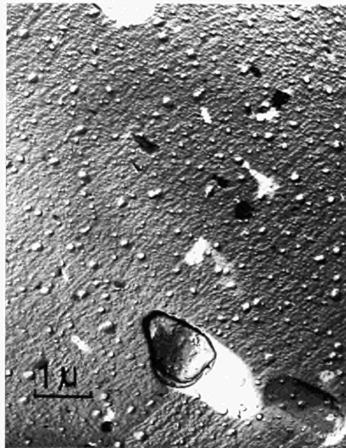
Fig. 16 : Artifacts due to non-dried triafol stripping
