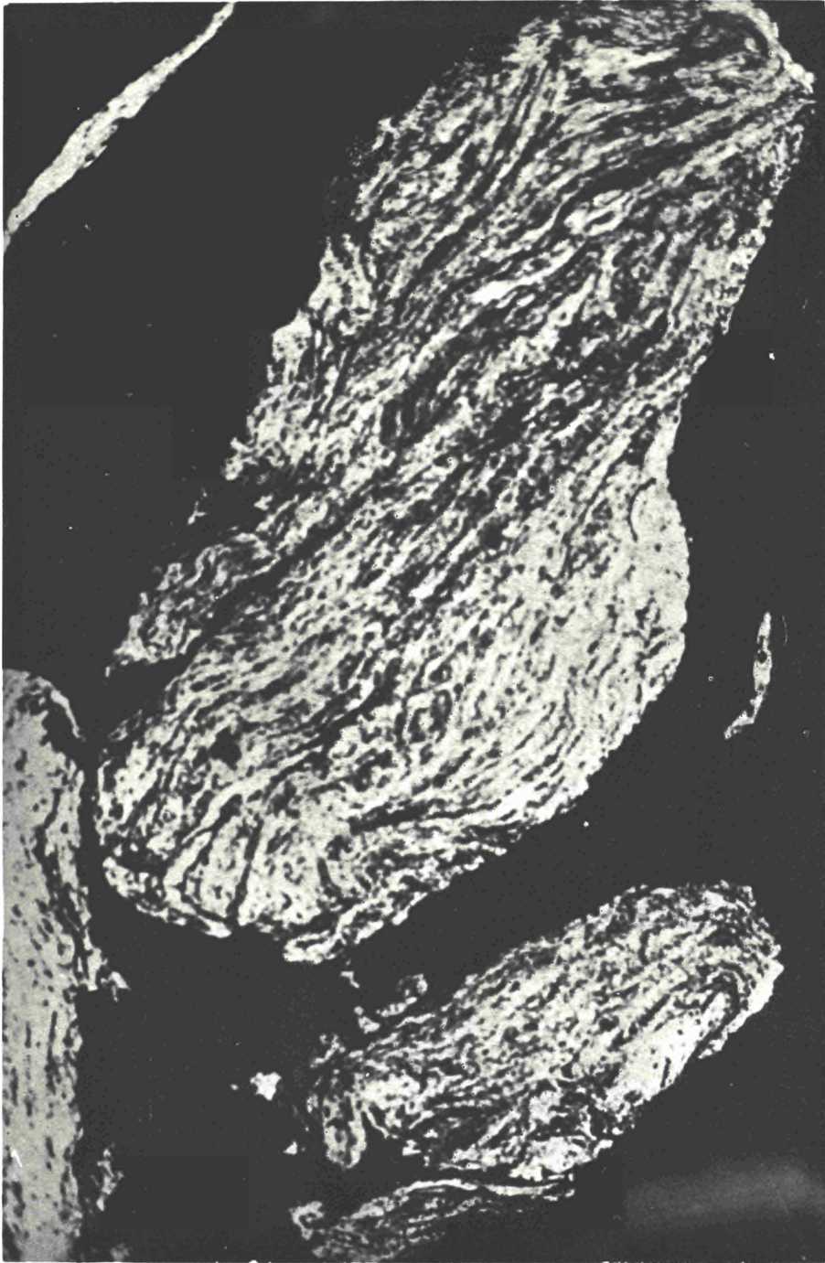
Illustration 1 Structural aspect of Al-Al 2 O 3 powders grade 960 Etching HF 0.5% Magnification 500 x
