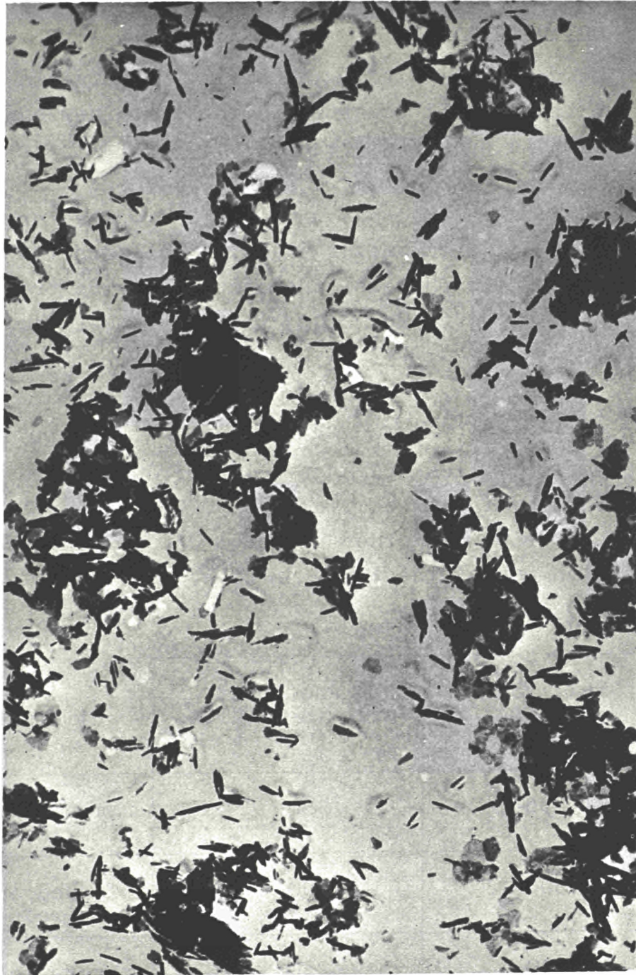
Illustration 4 Electron micrograph of a bar of SAP-ISML 7% \text{Al}_2\text{O}_3 Electron microscope magnifica- tion x 8,000 Total magnification x 20,000
