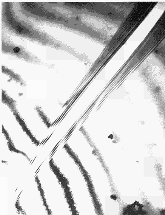
Fig. 2. A domain in a crystal wedge showing thickness fringes. The displacement of the thickness fringes in the domain is indicated by a local stronger contrast in the fringes of the domain boundaries.
