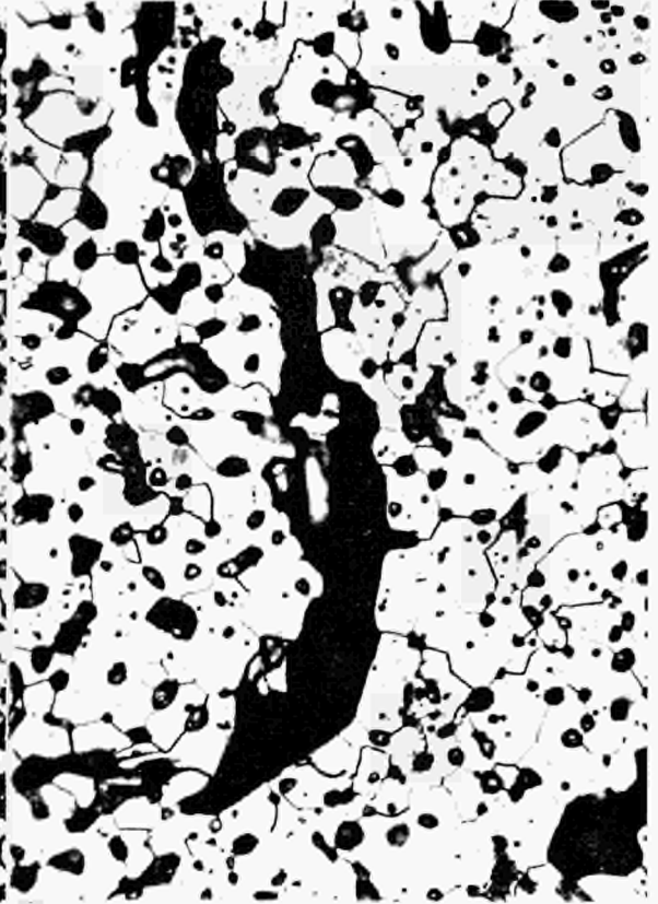
Fig. 3. Cavity formation during solarization. Soaking time: 5 h, T.D. 82.0 % etched. \times 1000
