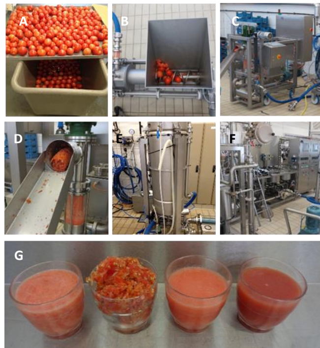
Figure 6.3 Tomato processing: A) washing, B) milling, C) pressing with spiral-filter press into D) press residue and E) juice, F) thermal pasteurization and G) resulting products, i.e. mashed tomato, press residue, non thermally treated tomato juice, thermally treated tomato juice.
