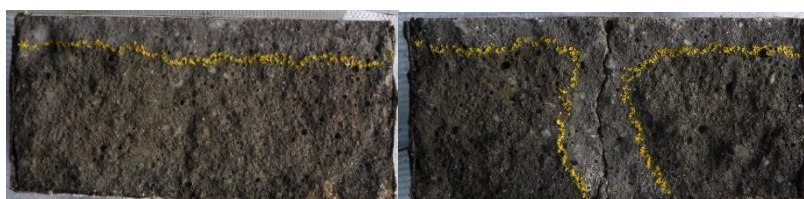
Figure 2: Chloride penetration in autogenously healed mortar with a remaining crack width < 10 \mu\text{m} (left) and > 10 \mu\text{m} (right) [adapted from 1]
