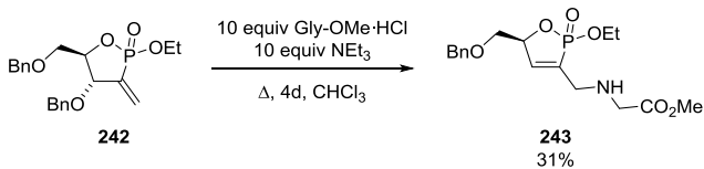
Scheme 57: \text{S}_{\text{N}}2' substitution reaction on phospho-1-oxo-pentofuranoses by glycine methyl ester.
