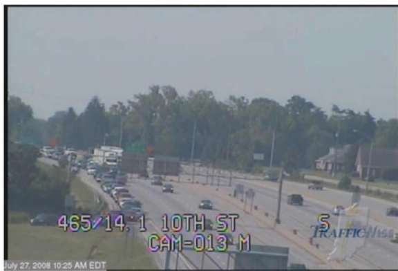
(a) 10:25 am. Ramp queue causing 2-mile backup on I-465 across three lanes.
