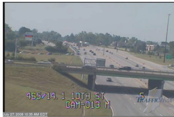
(b) 10:35 am. Northbound I-465 flow highly restricted by the exit ramp queue.
