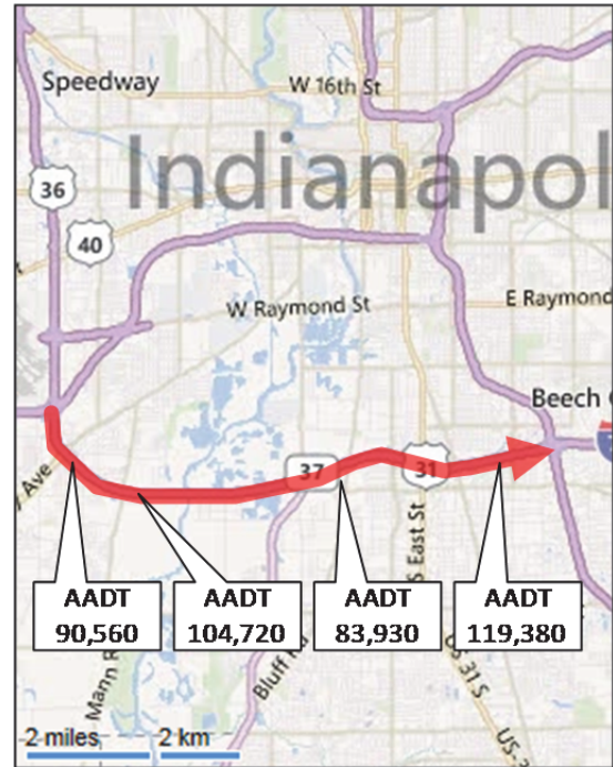
Figure C.86. Location of I-465 outer loop segment southwest of Indianapolis. (Table 5, Commuter Corridor Code I-12)
