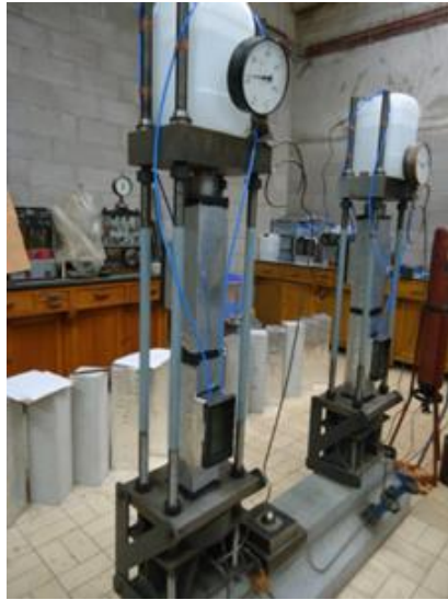
Figure 6-2: Two coaxially loaded prisms showing detail of the chloride stock solution and the loading rigs
