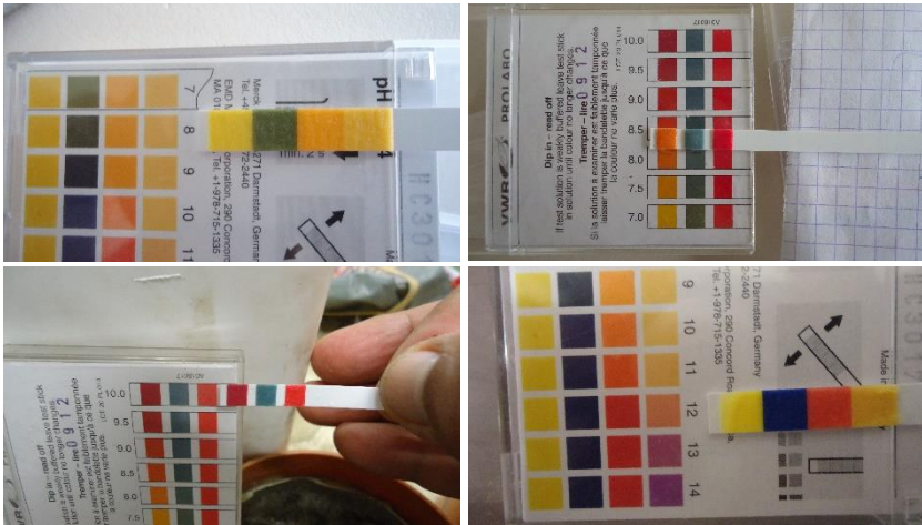
Figure 4-5: pH remaining levels in the attack solution after the last defrost cycle (56 days). For S70 (upper left), S50 (upper right), S0 (lower left) and HSR (Lower right).
