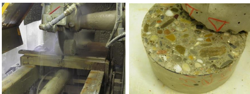
Figure 3-4: Cylinder cutting operation. One half of the cylinder is used to characterize carbonation depth, the other half for frost scaling studies on the remaining carbonated face.
