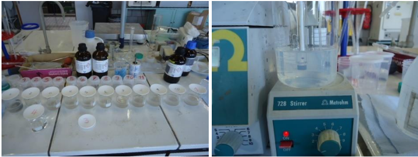
Figure 6-6: Extracted chloride solution from powdered samples with nitric acid digestion (left). Potentiometric titration of chloride with 0.01 M silver nitrate (right).
