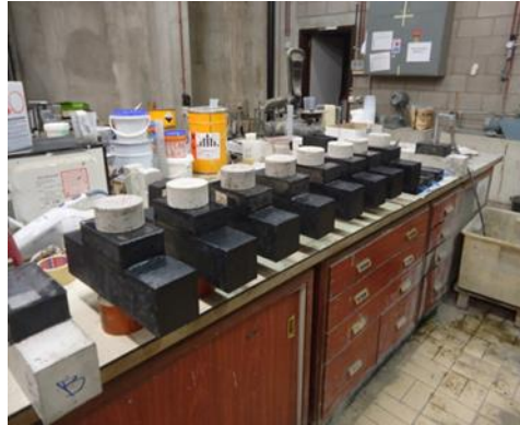
Figure 6-1: Concrete prisms with the solution tank and covered with black silicon to impermeabilize the sample.
