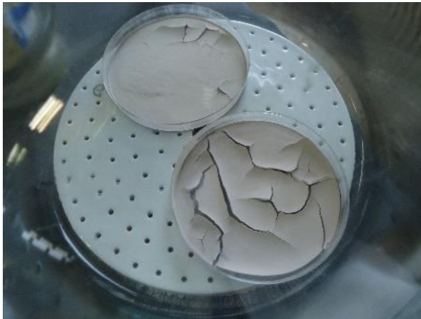
Figure 3-7: Extracted cement paste from concrete, for XRD analysis.
