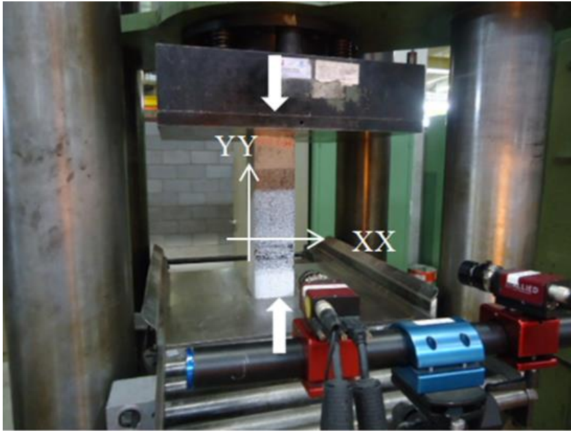
Figure 6-3: Prismatic samples with the digital image correlation (DIC) pattern setup.
