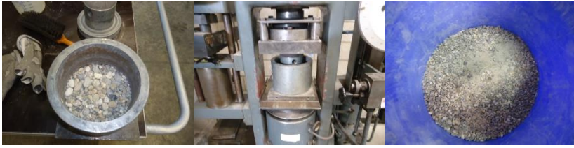
Figure 2-2: Preparation of aggregate composition for mineral analysis with XRD.
