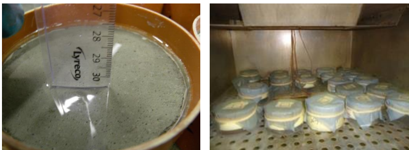
Figure 4-2: Chloride solution ponding (left). Concrete samples in freeze and thaw chamber (right).
