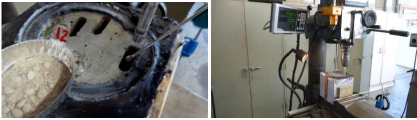
Figure 6-23: 10 mm wide by 30 mm long grooves for chloride powder extraction (left). Detail of the drilling tool provided with sliding table in 2 directions (right).
