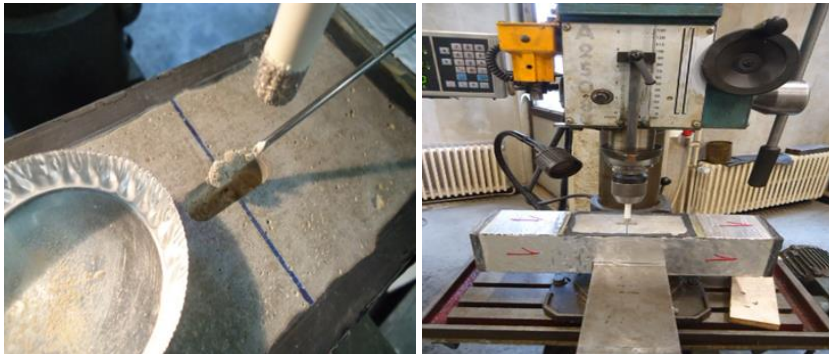
Figure 6-5: 10 mm wide by 30 mm long grooves for chloride powder extraction (left). Detail of the drilling tool provided with sliding table in 2 directions (right)
