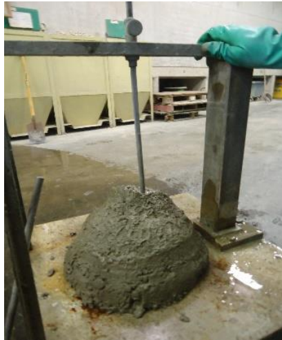
Figure 2-4: Fresh concrete slump test. Concrete slump class S4 (160-210 mm).
