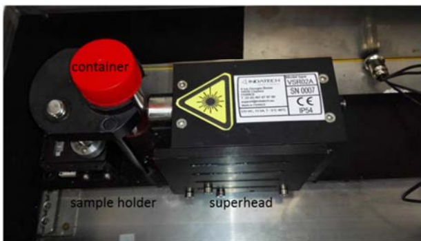
Fig. 1. Experimental set-up: A. Raman superhead enclosed in metal box, with sample in plastic container ready for measurement. B. Content of box: fiber-optic Raman probe facing the sample holder. C. Branch of the production line passing through the lab for sample collection.
