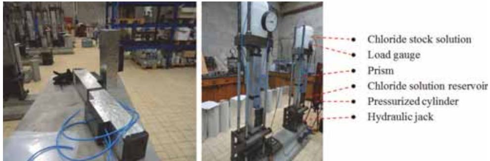
Figure 2. Setup for combined chloride attack (2 prism), plus compressive loading.
