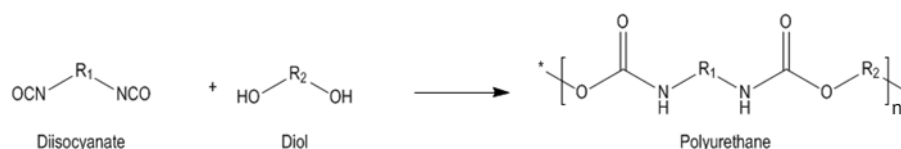
Figure 2: General synthesis scheme for a linear polyurethane based on a diol and a diisocyanate.
