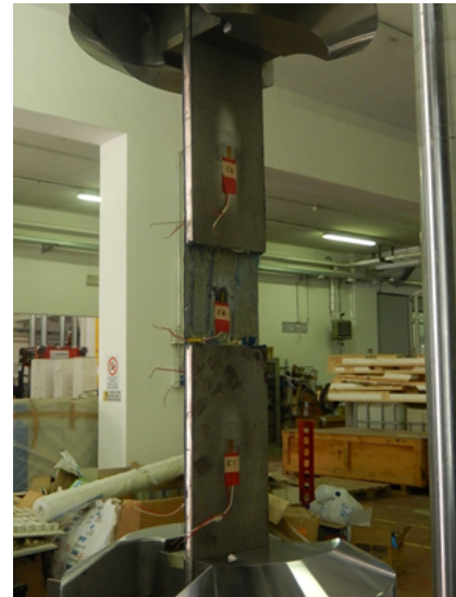
(b) Specimen S1 after delamination.
