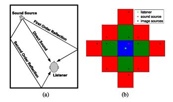
Figure 1: (a) Sound path in a room. (b) 2D schematization of the image-sources method. The simulated room is in blue, first order reflections are located in green areas and second order reflections are located in red areas. The listener is a green  $\bullet$ , the source a red  $\bullet$ .
