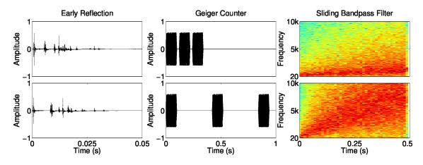
Figure 2: Representation of the sound resulting from the application of the three effect metaphors for two distances: top = 0.6 m, bottom = 1.5 m; (Left) Impulse response of the Early Reflection effect metaphor. (Center) Geiger Counter effect metaphor applied to a 10 ms burst. (Right) Spectrogram of the sounds resulting from the Sliding Bandpass Filter effect metaphor applied to a 0.5 sec burst.
