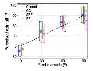
Figure 7: (a) Perceived azimuth as a function of rendered azimuth for each sonification condition.  $\ll \Box$ ,  $\triangle$ ,  $\circ$ ,  $\times \gg$ : Mean for each condition. Vertical lines: Standard deviation for each modality. For the sake of readability, results corresponding to the different conditions have been slightly horizontally shifted.
