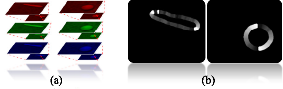
Figure 5: (a) Gaussian Pyramids on red, green and blue channels. (b) Gabor Transform response images.
