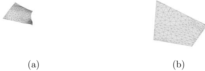
Fig. 25. Illustration of parameterization. (a) One of four patches in Fig. 24(c). (b) The polygonal domain and its parameterization mapping.
