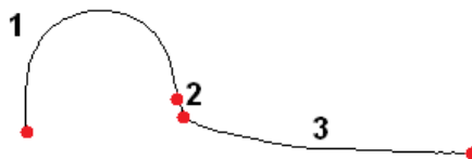
Fig. 32. Initial set of corners found for a stroke consisting of an arc and a line. Segment 2 is the smallest, unneeded segment and should be merged with Segment 1.
