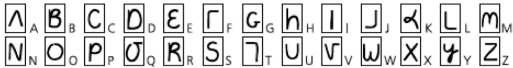
Fig. 8. Palm’s Graffiti gesture system allowed users to write on a PDA with a stylus and achieve high recognition results. The gesture language mapped well to Roman characters, and the single-stroke recognition allowed Palm devices to quickly and accurately classify each stroke [14].
