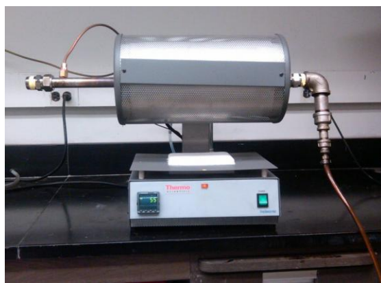
Figure 3. Tube furnace used for fixed-bed, slow pyrolysis experiments.
