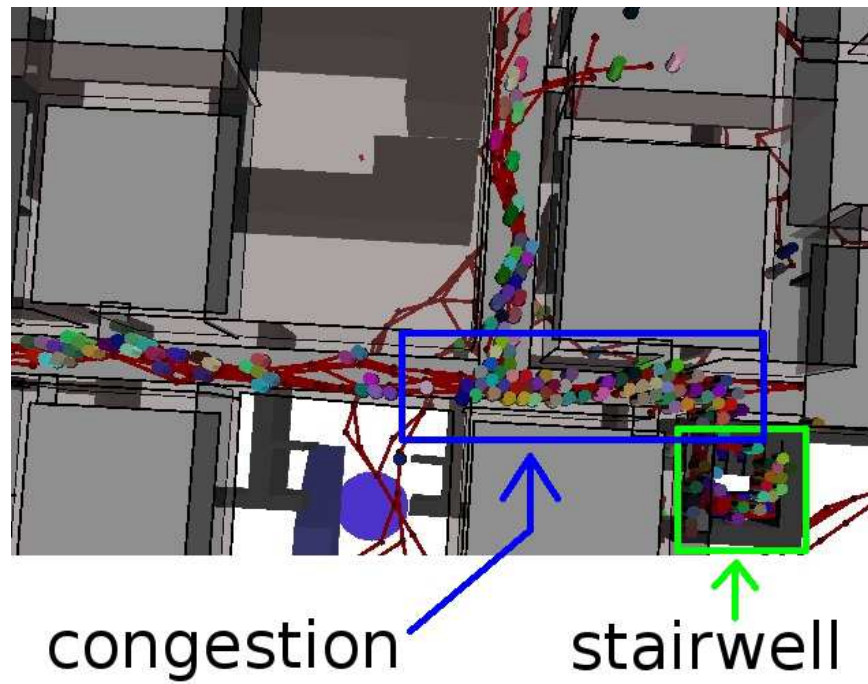
Figure 41: Congestion occurring before agents enter stairwell. This congestion is in part due to agents having to organize themselves before traveling through the available stairwell.
