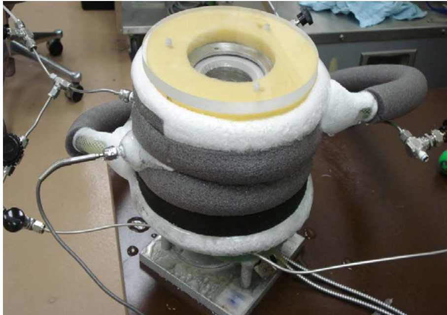
Fig. 19 High pressure stainless steel cell used for formation and decomposition of gas hydrates.
