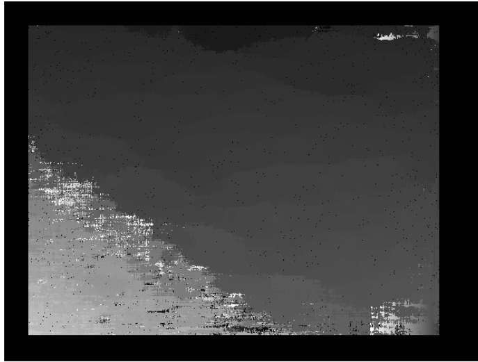
Fig. 14. 2-Dimensional implementation, resulting raw disparity map.
