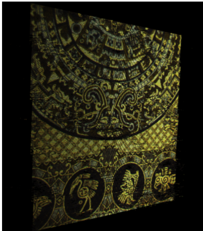
Fig. 35. Three dimensional reconstruction generated by CUDA phase based dense stereo algorithm, from nearly fronto-parallel Mayan blanket plane scene.
