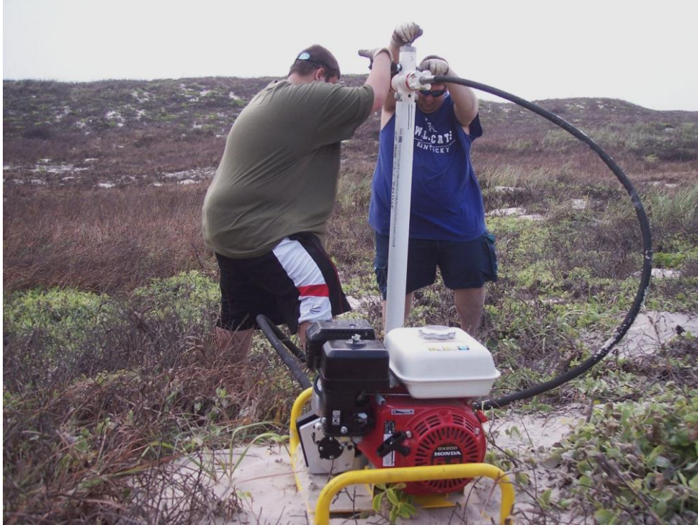
Figure 11. Modified vibra-coring system accommodating 3-inch-diameter PVC pipe.
