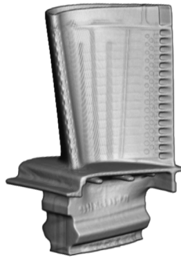
Fig. 16.: Schematic of a turbine blade with a pin fin cooling array in the trailing edge region from Kindlmann (1999) [18].
