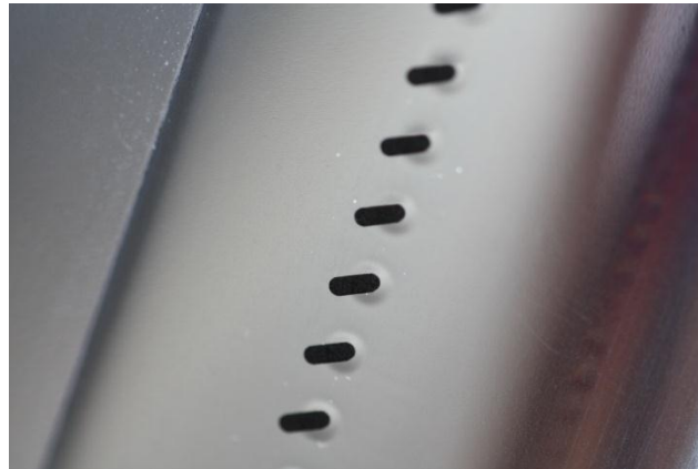
Figure 31: Appliqué DREs superposed on pneumatic DREs
