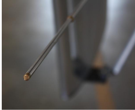
Figure 26: Five-hole probe attached to the SWIFT model
