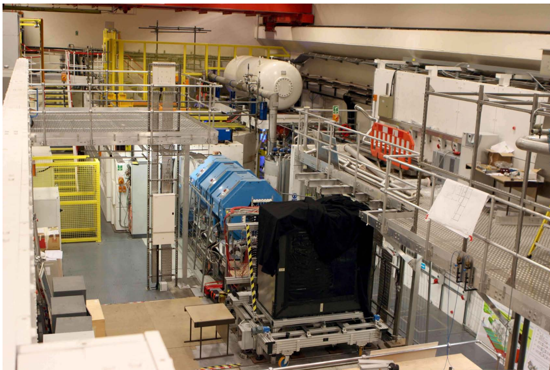
Figure 9. Downstream beam line. The ISIS synchrotron lies behind the curved wall in the background. The downstream quadrupoles (blue, hexagonal magnets) may be seen just downstream of the white concrete shielding. The time-of-flight counter TOF1 is seen immediately downstream of the final quadrupole. TOF1 is followed by the KL and the prototype EMR.
