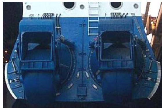
(b) Interceptor steering system on Stena HSS
