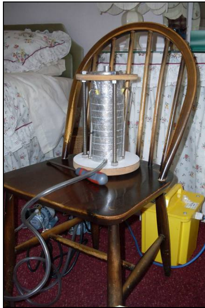
Figure 5-13: Andersen Sampler was placed about 1m from floor level
