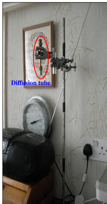
Figure 4-4: The open end of diffusion tube was held vertically facing downwards
