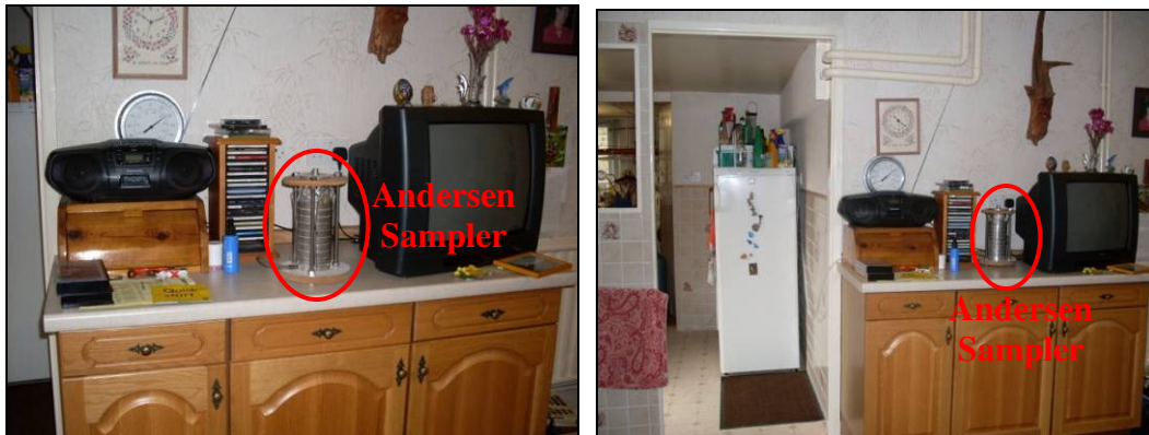
Figure 5-25: The Andersen Sampler was placed about 1.5m from floor level
