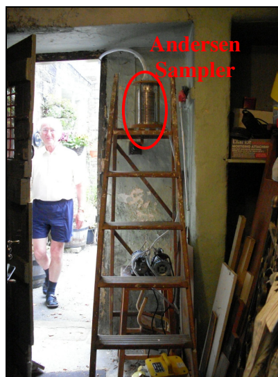
Figure 5-51: The Andersen Sampler was placed about 2.0m from floor level
