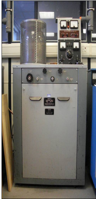
Figure 4-3: Edwards Carbon Coating Unit (Model: 12E6/1598)
