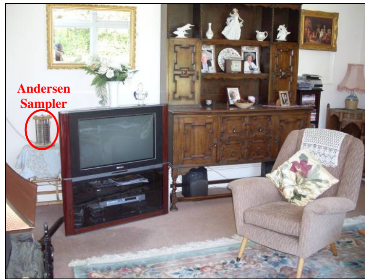
Figure 5-39: The Andersen Sampler was placed about 0.8m from floor level
