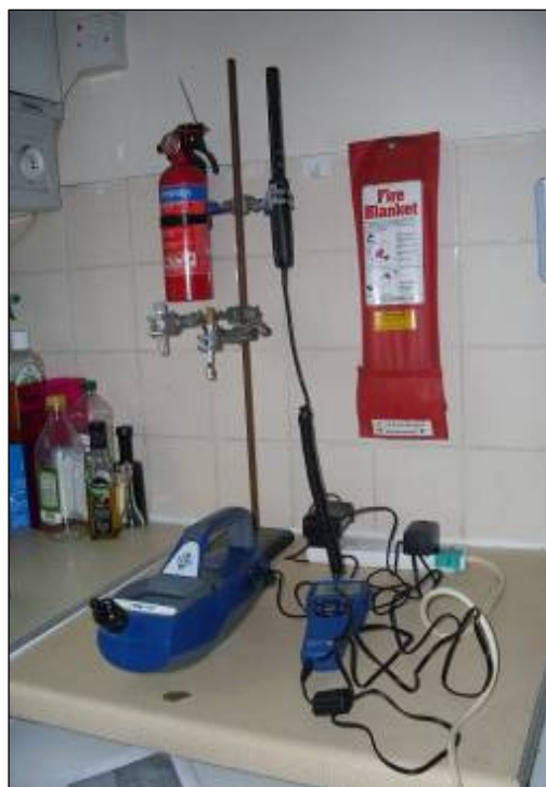
Figure 7-8: Installation of sampling equipment inside the kitchen
