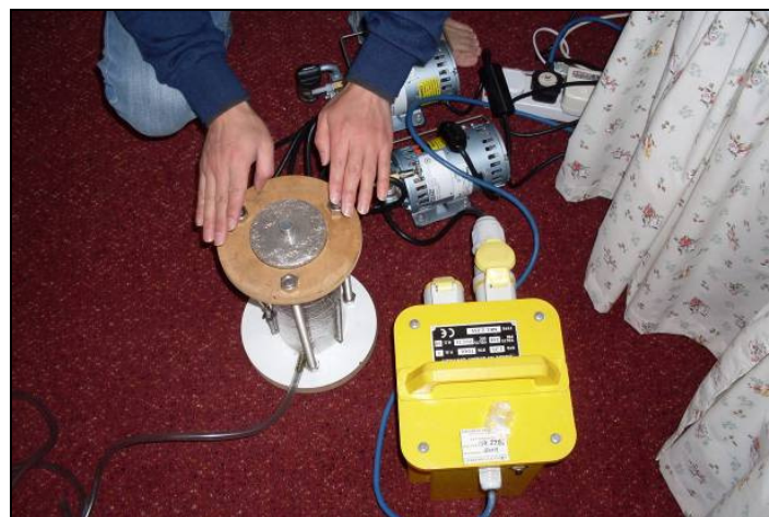
Figure 5-12: Installation of Andersen Sampler
