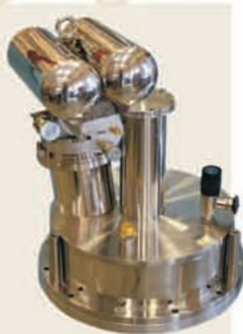
The prototype cryo-free system based on the PTR for providing cryogenic sample environment for neutron scattering experiments.
