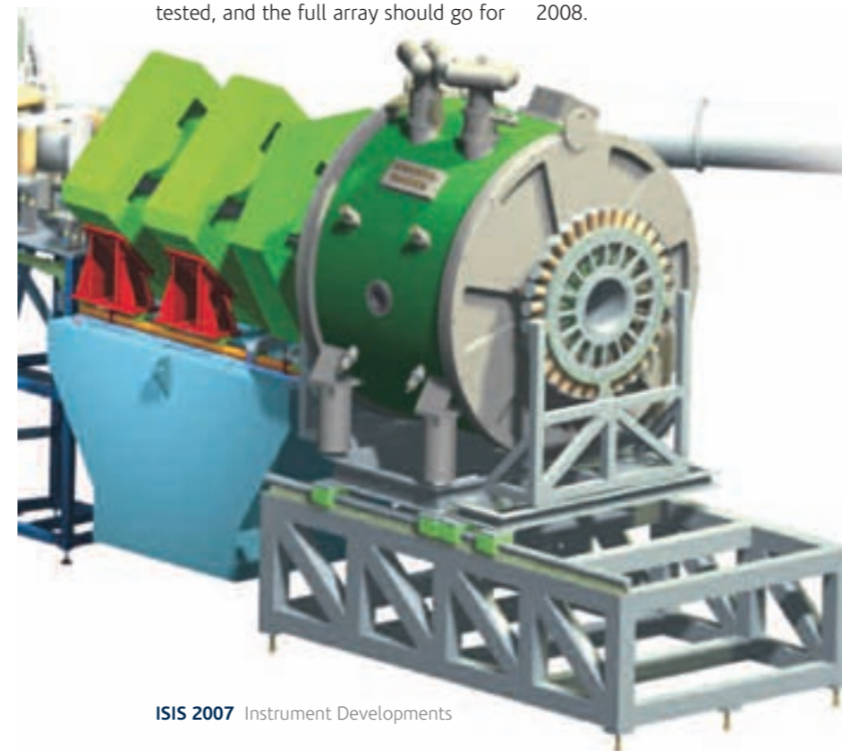
Schematic of the new Hifi muon spectrometer, showing the 5T superconducting magnet, instrument detector array and beamline.
